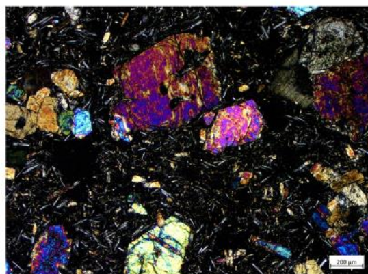
Figure 2. A photomicrograph of a representative Lung Po Pleistocene alkaline basalt shows euhedral and subhedral olivine phenocrysts on a holohyaline groundmass with plagioclase microlite and Fe-Ti oxides; the left photo is taken under plain light, and the right photo is taken under polarized light
