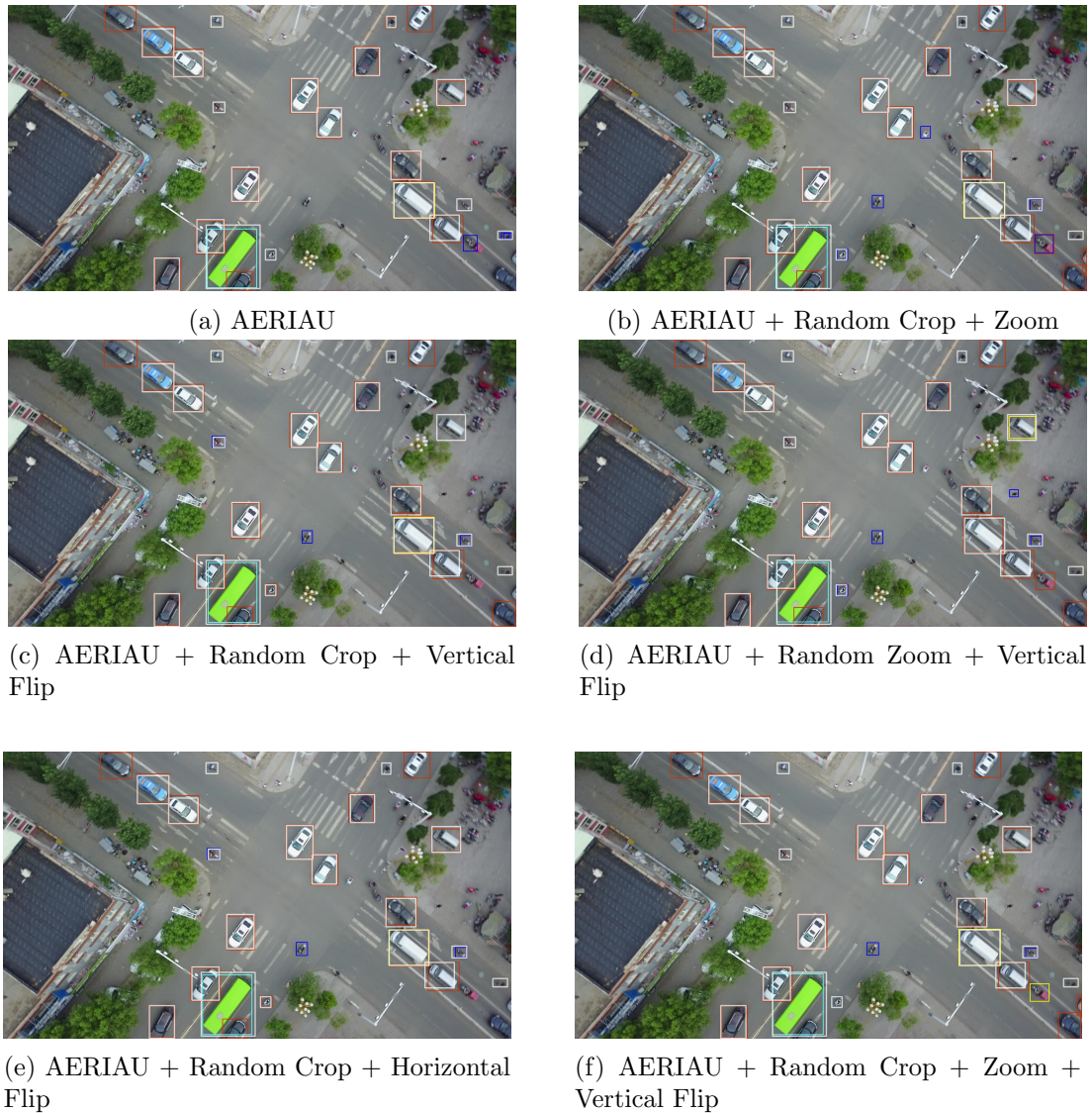
Figure 6: Faster RCNN: Visualization results of Combined Data Augmentation Strategies. Color legend: truck, car, bus, motor, and Ground Truth.
