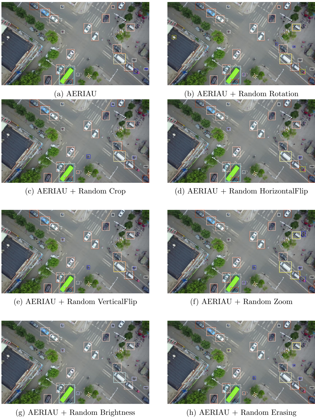
Figure 5: Faster RCNN: Visualization results of Single Data Augmentation Strategies. Color legend: truck, car, bus, motor, and Ground Truth.
