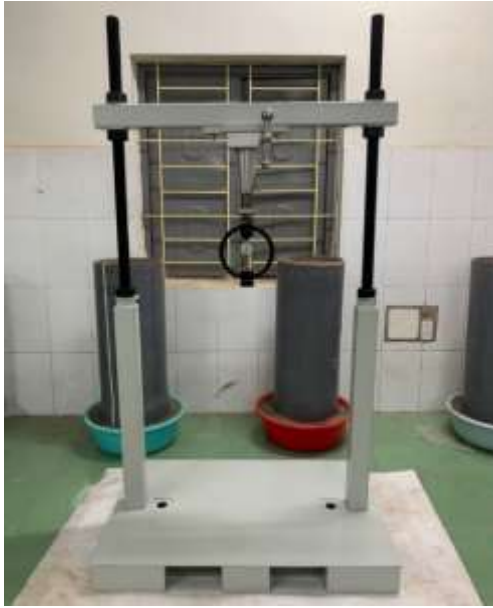
Figure 6. Loading frame system for single stone column
