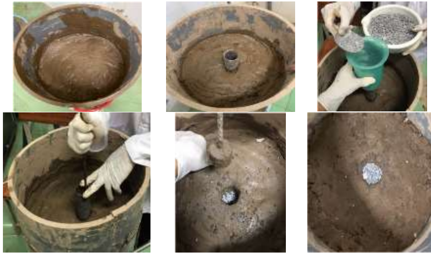
Figure 7. Steps to create a single stone column in the experimental model
