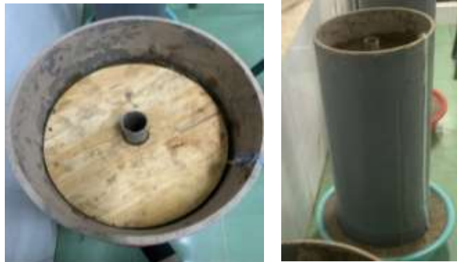
Figure 5. Test tank made of composite pipe
