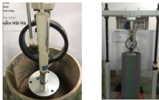
Figure 8. Displacement and load measuring system in a single-stone column experimental model
